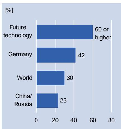
**Figure 14:** Efficiency of hard-coal power plants, Source: GVSt
