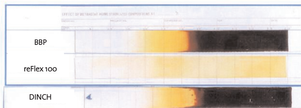
Figure 5 Improved thermal stability of reFlex™ 100, a bio-derived green plasticizer, compared to butyl benzyl Phthalate (BBP) plasticizer, and diisononylcyclohexane-1,2 dicarboxylate (DINCH), a petroleum-based non-phthalate plasticizer. Test conducted on heat stability in a metastat oven set to 375 degrees for 5-to-60 minutes.
